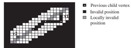
Figure 6. Dynamically reduced set of positions for child vertices along a level 2 parent edge, 3 previously transmitted child vertices, geometrical rules (5,6,7).
